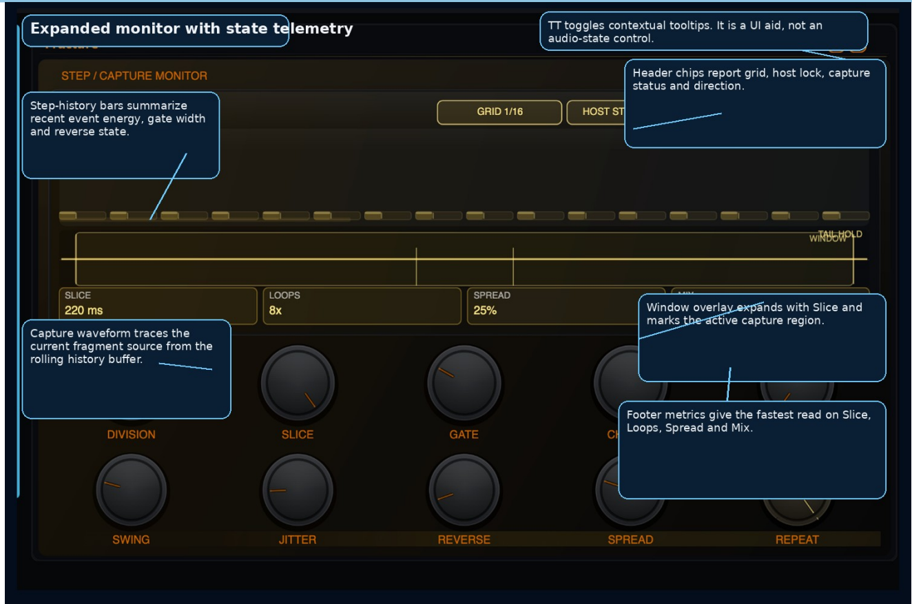
Figure 4. Expanded monitor, showing the step-history bars, capture waveform, playback window, header state chips and footer metrics.
