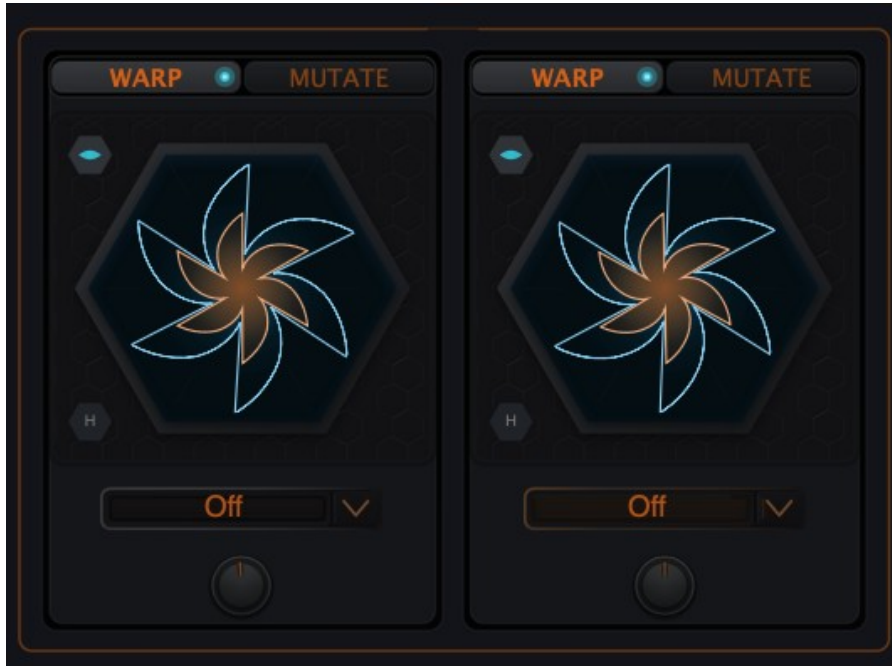
Figure 3. Prism Core in neutral/off state. The two tabs select Warp or Mutate for each oscillator.
