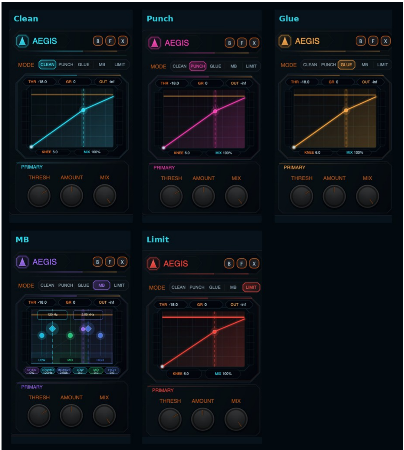
Figure 2. Compact card states: Clean, Punch, Glue, MB, and Limit. Compact view keeps Threshold, Amount, and Mix close while condensing the shield screen.
