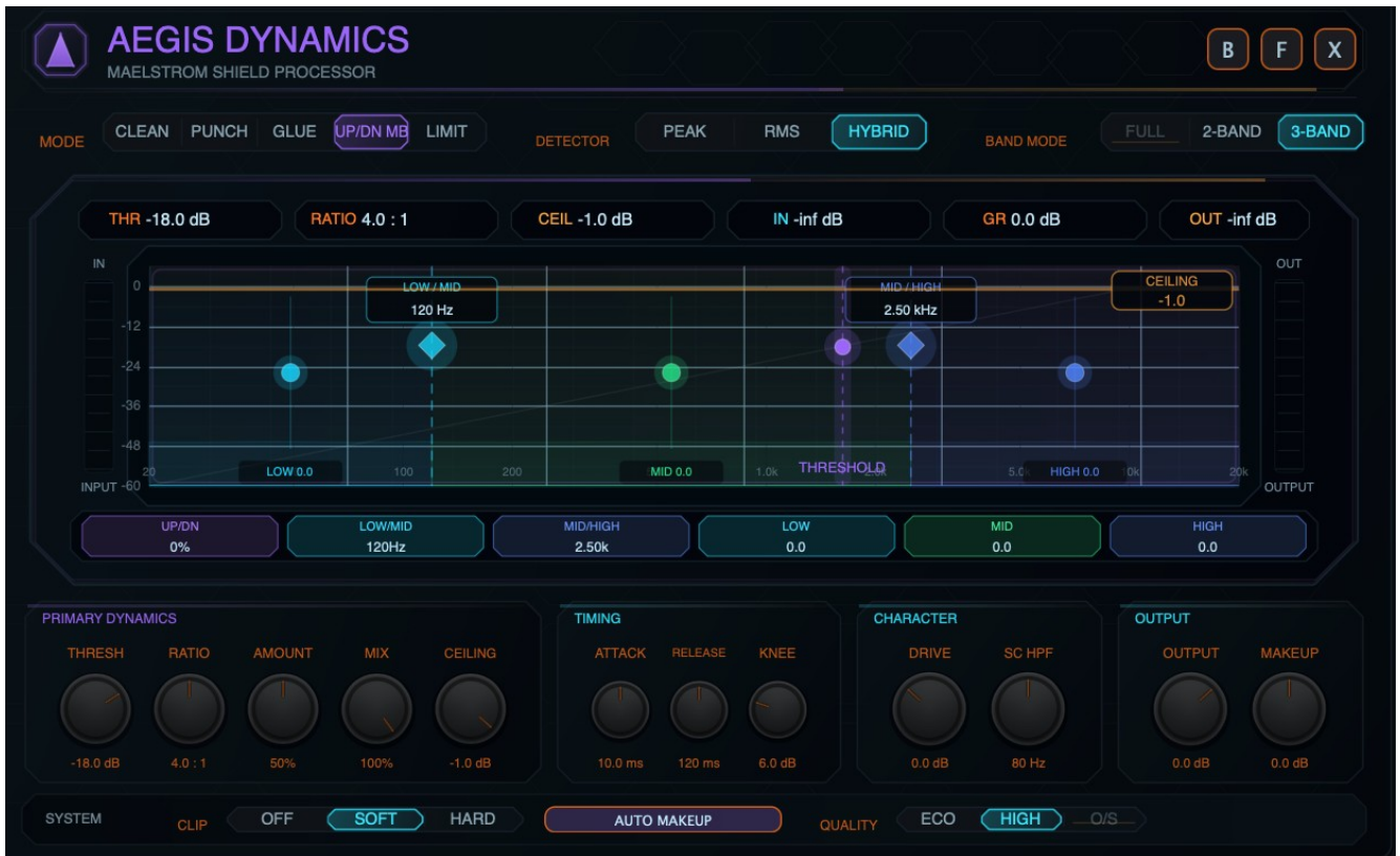
Figure 7. Up/Dn MB in 3-Band mode. Full is disabled, multiband controls are active, and O/S is unavailable in multiband operation.
