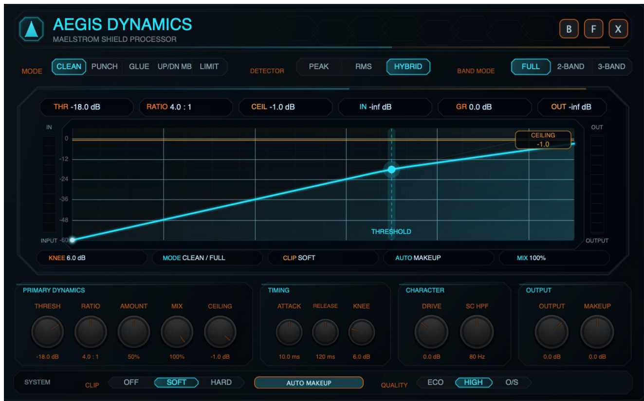
Figure 3. Expanded Clean / Full view, showing the transfer curve, threshold handle, ceiling rail, lower rail, and Quality strip.
