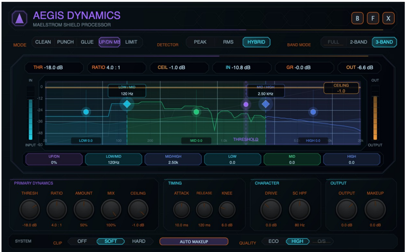
Figure 10. Live multiband visualizer with spectrum trace, crossover handles, trim handles, threshold, ceiling, and meters.
