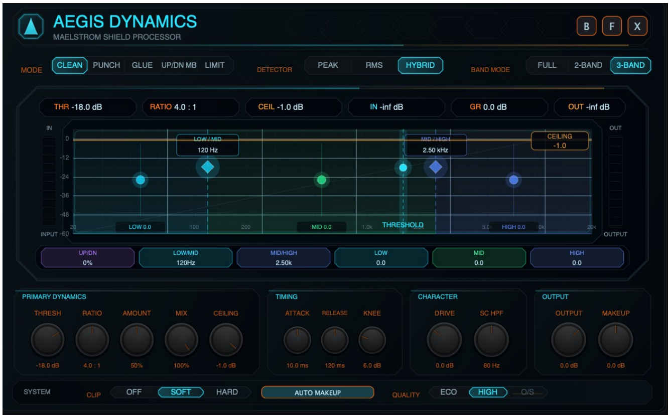
Figure 9. Clean / 3-Band view, showing Low, Mid, and High regions plus Low/Mid and Mid/High crossover controls.
