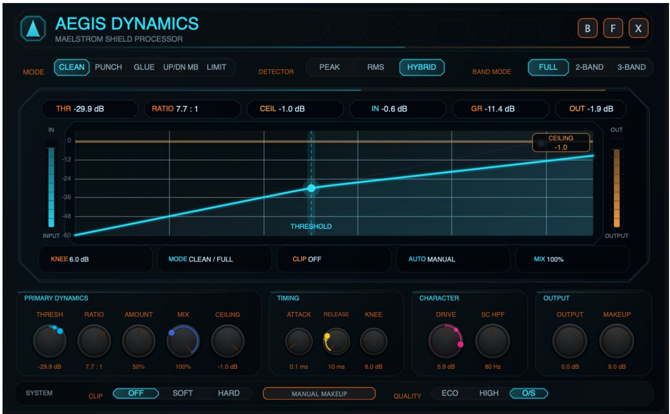
Figure 11. Live input, gain-reduction, and output readouts in expanded Full mode.
