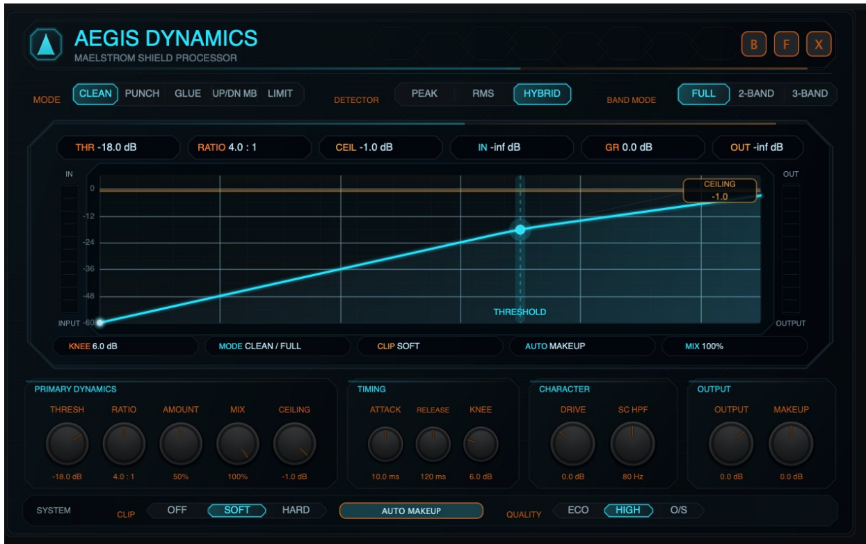
Figure 13. Expanded Aegis Dynamics editor with mode strip, detector, band mode, transfer display and dynamics controls.
